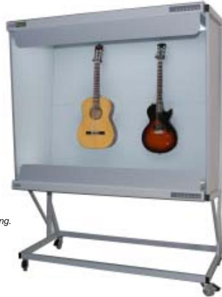
The VCMB-64 (at right) is used to evaluate finish details for wood coating.
