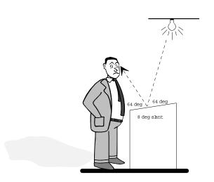
The source of the light has been moved to behind the observer's head. Now the reflection off the viewing surface is away from the observer's eye, and glare is eliminated.
