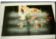
Improper geometry - excessive glare
