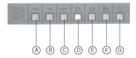
Press and hold the SEQ "A" button. While holding the SEQ button, press the buttons for the sources you wish to turn on in the order you want them activated (up to 10). After selecting your light sources, while still holding the SEQ button, press the Power "G" button for the length of time you want each source to be on.
