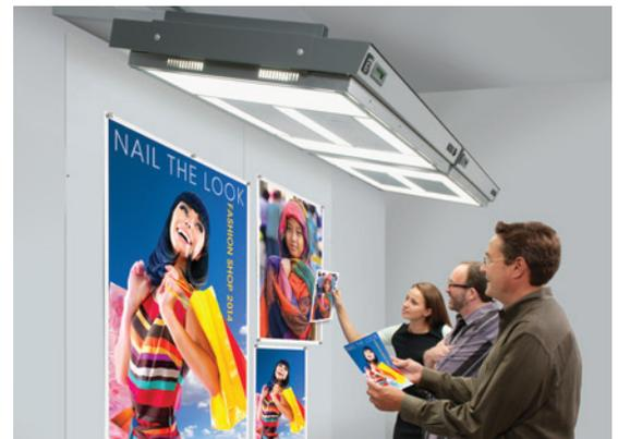
**When D50 or D65 standard illumination is reflected from colored walls its color quality changes so it is no longer “standard”. The application of a neutral gray paint to surrounding surfaces will eliminate this color pollution by providing spectrally neutral surfaces around the viewing area.**
