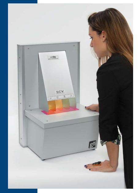
Above: The SCV Simultaneous Color Viewer facilitates accurate color viewing and detection of metamerism, the condition when colored objects match in one light source but not in another.
