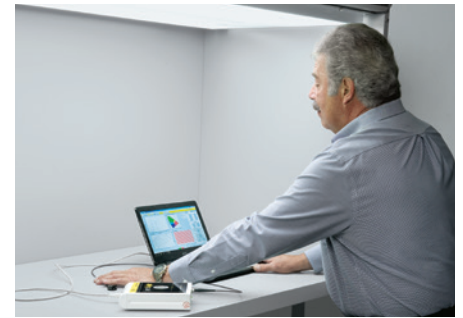
Verifying conformance with a spectroradiometer.
