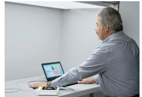
Verifying conformance with a spectroradiometer.
