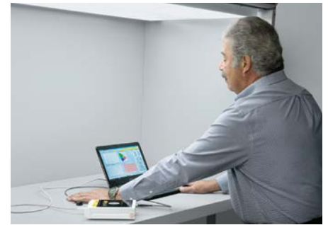
Verifying conformance with a spectroradiometer.
